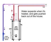
Once the backflow assembly in installed, the water can no longer expand into the public water supply and relieve this pressure. Therefore, pressure on the house plumbing can increase dramatically.
