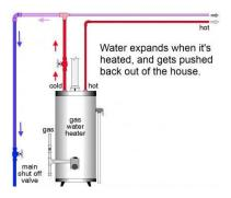
Once the backflow assembly is installed, the water can no longer expand into the public water supply and relieve this pressure. Therefore, pressure on the house plumbing can increase dramatically.
